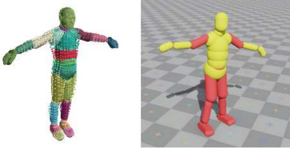
Fig. 4. Left: Physical character model defined by optimizing rigid body geometry (colored volumes) to match a human character mesh (colored points) based on the motion capture actor. Right: Feedback policy only provides actions that alter actuation of a subset of bodies (red). Other bodies (yellow) are driven purely by open-loop control.
